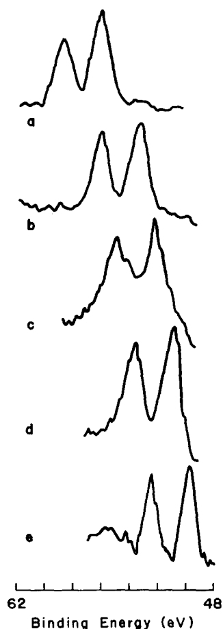
Fig. 1. ESCA spectra of the 4 f electrons of osmium in various oxidation states: (a) Os(VIII), OsO 4 ; (b) Os(VI), K 2 OsO 2 (OH) 4 ; (c) Os(IV), K 2 OsCl 6 ; (d) Os(III), OsCl 3 ; and (e) Os(II), K 4 Os(CN) 6 .
